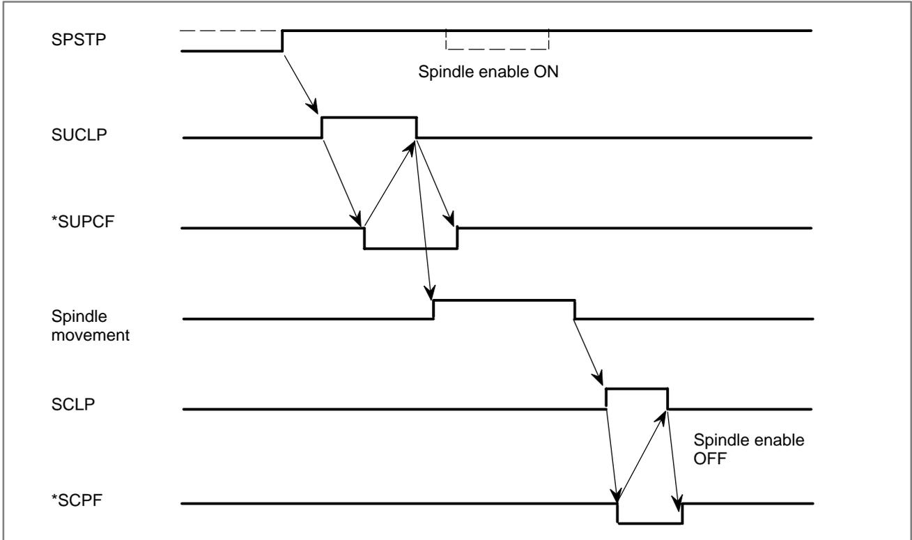
**Spindle Positioning Reset**
