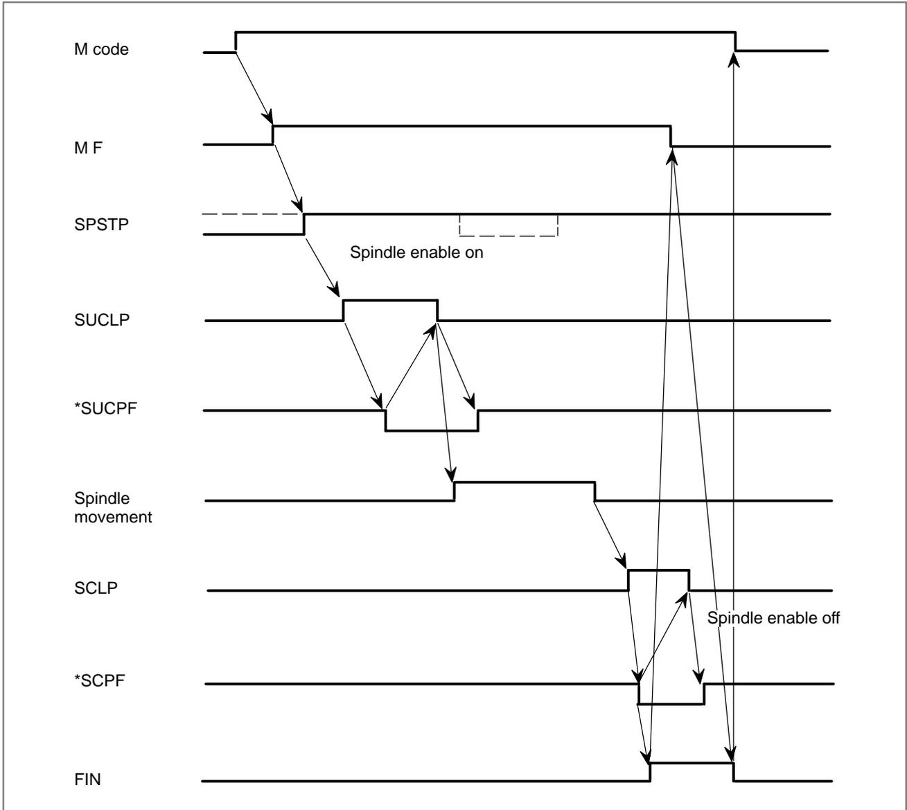
**Spindle Positioning by Address C,H**
