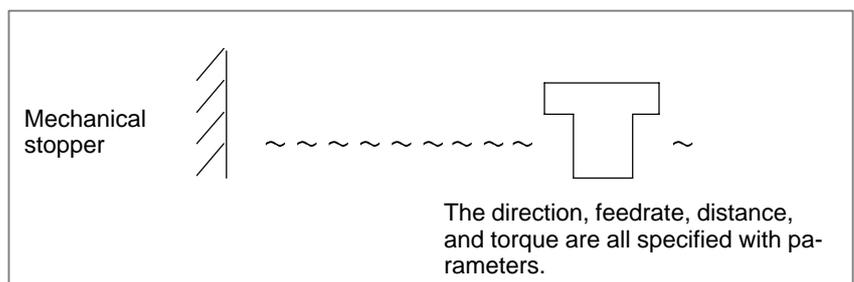
(C) Operations (D) and (E) are performed from the withdrawal point, such that the tool is butted against the mechanical stopper at a constant feedrate in reference position setting.
