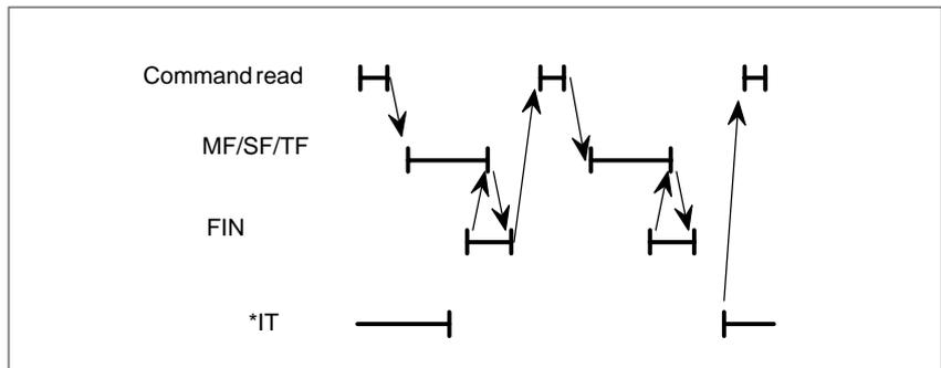
**Fig. 2.5 (d) Block containing auxiliary functions only (automatic operation)****NOTE**
