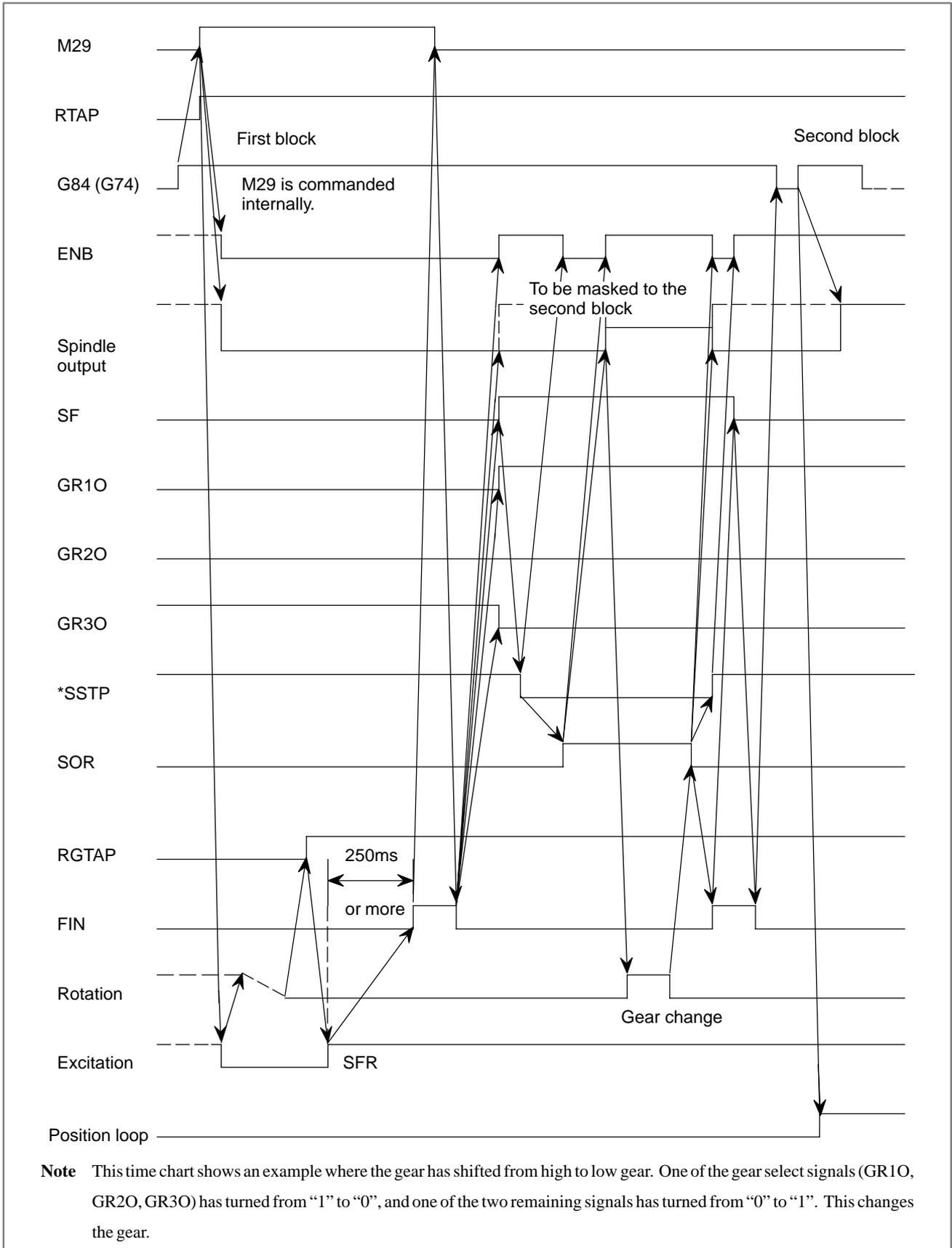
Fig. 9.10.7.3 (b) When gear change is performed (high to low gear)
