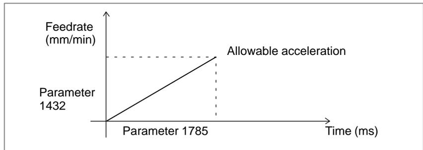
● **Parameters related to feedrate clamping by arc radius**
