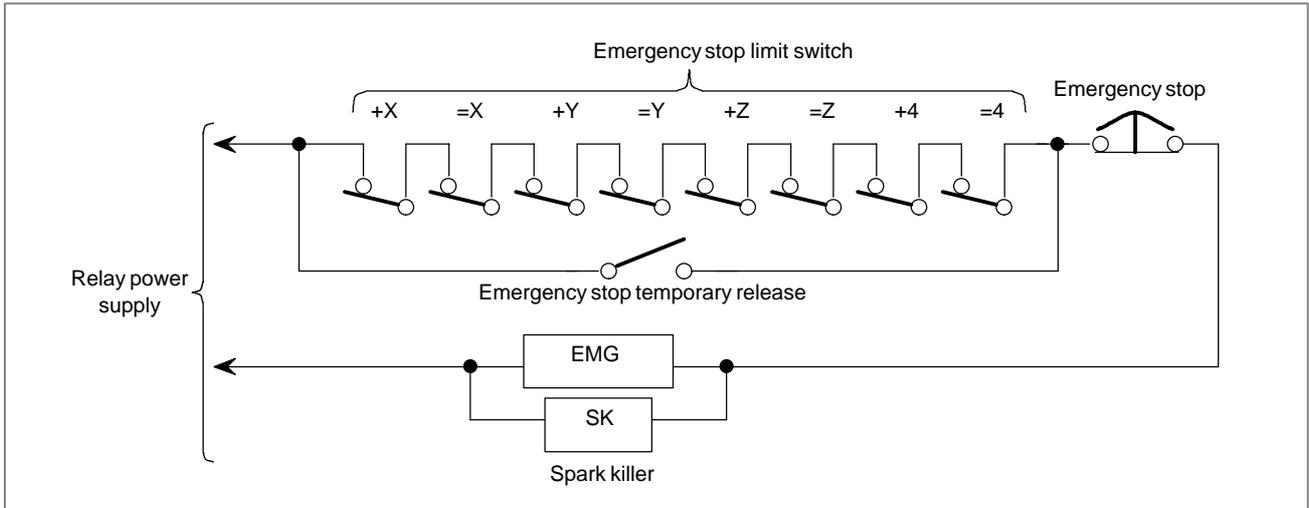
Fig. 2.1 (b) Connection of emergency stop limit switch
