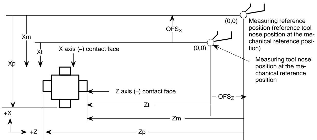
$X_P$  : Distance from the measuring reference position to X-axis (+) contact face (parameter no. 5015)
