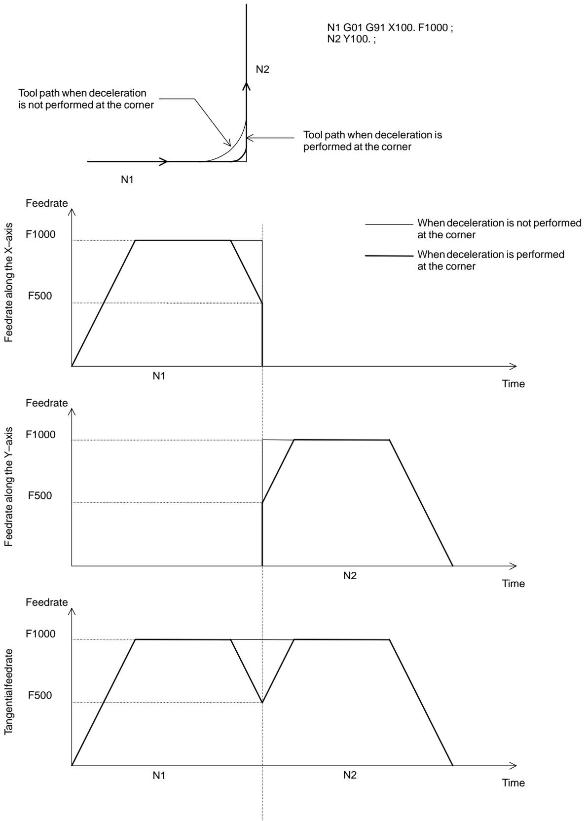
● **Feedrate clamping by acceleration**
