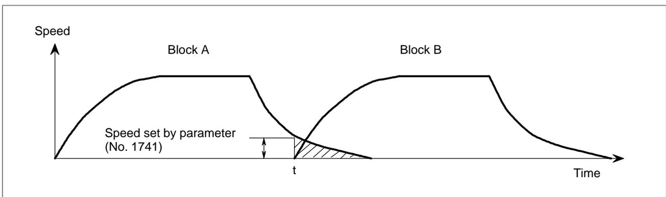
· **When linear acceleration/deceleration before interpolation for cutting feed is enabled**
