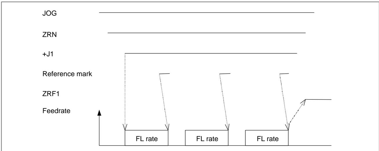
**Fig. 4.7(b) Timing chart for reference position establishment**
