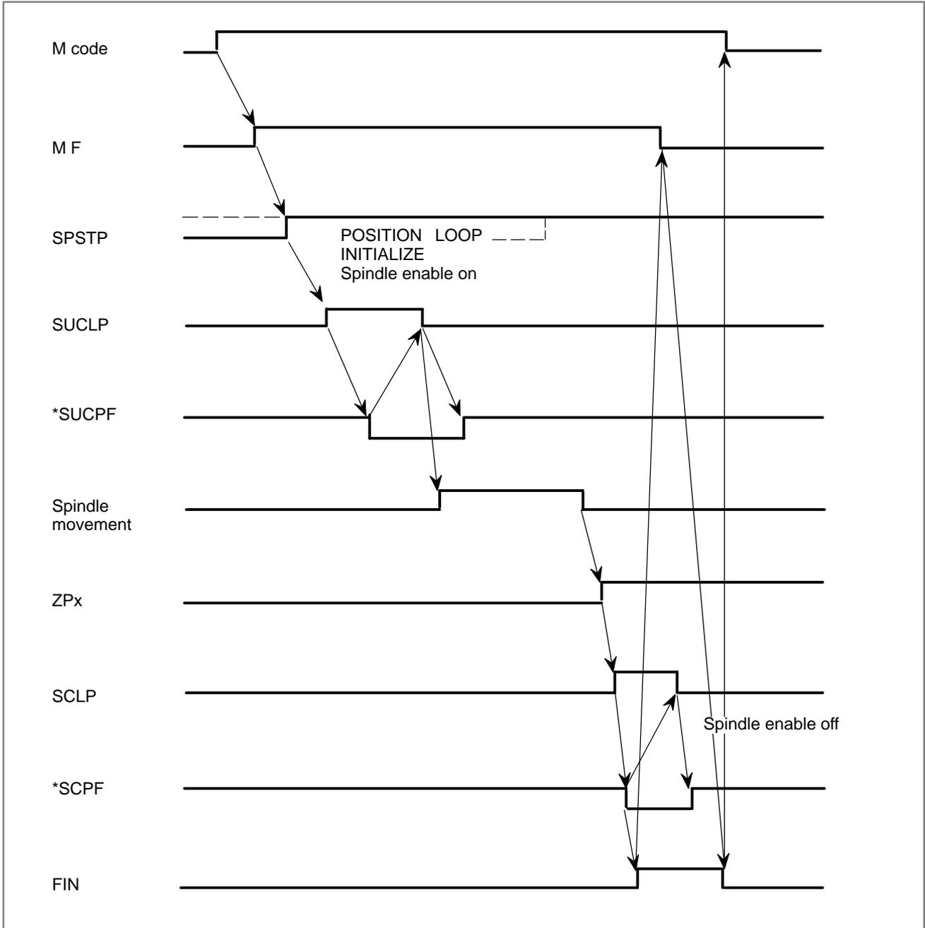
⇒ POSITION LOOP INITIALIZE is performed within the CNC.
