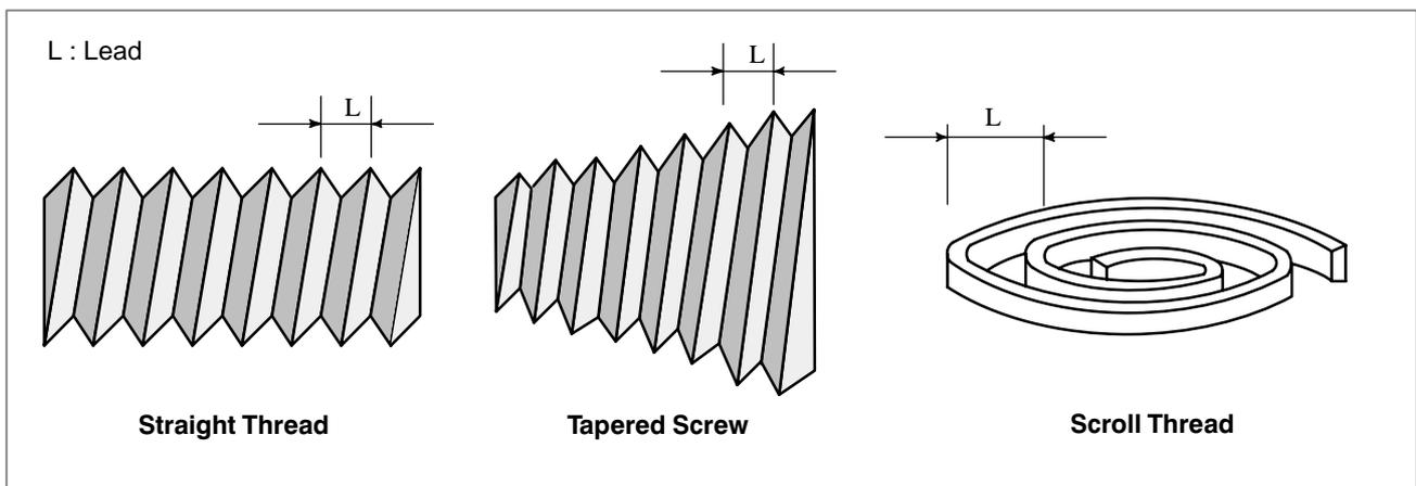
In general, thread cutting is repeated along the same tool path in rough cutting through finish cutting for a screw. Since thread cutting starts when the position coder mounted on the spindle outputs a 1-turn signal, threading is started at a fixed point and the tool path on the workpiece is unchanged for repeated thread cutting. Note that the spindle speed must remain constant from rough cutting through finish cutting. If not, incorrect thread lead will occur.
