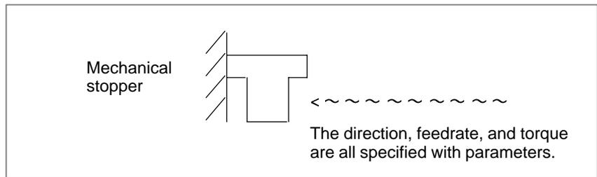
(E) After the tool strikes the mechanical stopper end on the axis, the tool is withdrawn in the direction opposite to the butting direction, along the axis for a parameter-set distance.
