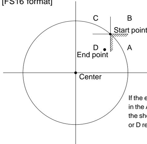
If the end point viewed from the start point is in the A region, the movement is made along the shortcut. If the end point is in the B, C, or D region, almost a single turn is made.
