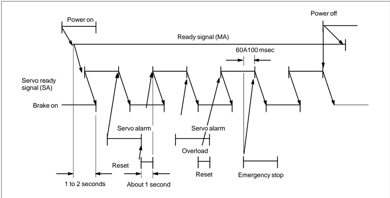
**Fig. 2.2 Time chart for servo ready signal**
