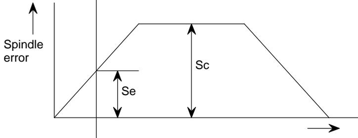
$$S_c = \frac{\text{Speed} \times 360}{60} \times \frac{1}{\text{Gain}} \times \frac{1}{\text{Detection unit}} \times 10^2 \text{ (Theoretical value)}$$
