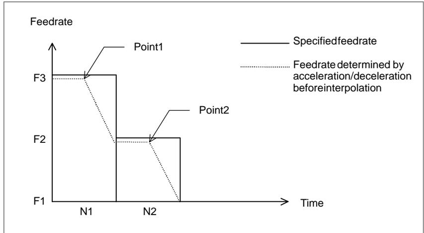
To decelerate from feedrate F3 to F2, deceleration must start with point 1. To decelerate from feedrate F2 to F1, deceleration must start with point 2.
