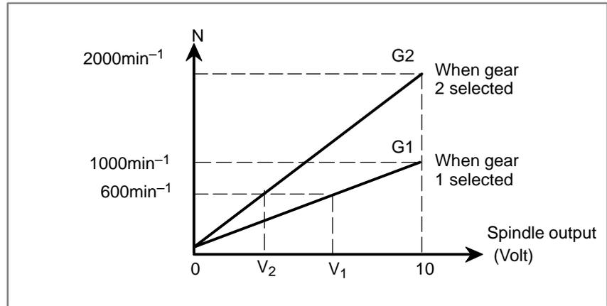
Here, S = 60 m/min is given as the surface speed; if the position of the present X-axis cutter is 16 mm from the center, the spindle speed N becomes 600 min<sup>-1</sup> (S = 2πr N). Therefore, V<sub>1</sub> (for G1) or V<sub>2</sub> (for G2) is calculated inside the CNC and output to the machine side.
