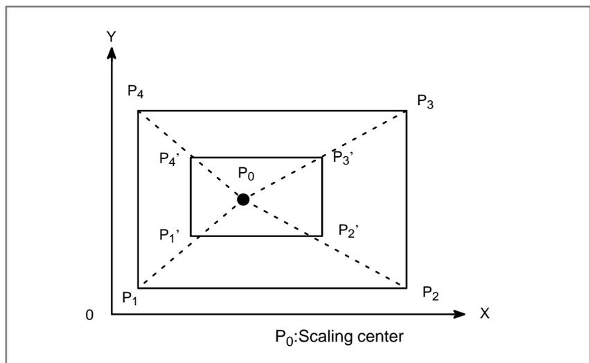
Fig. 11.11 (a) Scaling (P<sub>1</sub> P<sub>2</sub> P<sub>3</sub> P<sub>4</sub>→P<sub>1</sub>'P<sub>2</sub>'P<sub>3</sub>'P<sub>4</sub>')
