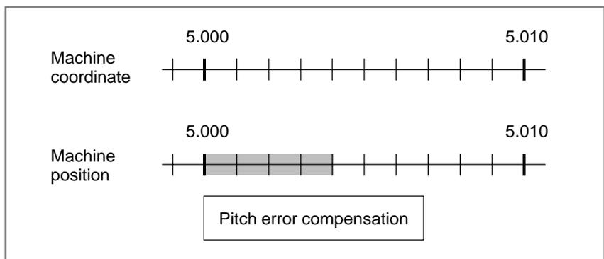
Assuming that a pitch error compensation of +0.004 is specified for a pitch error compensation interval of 10.000 degrees and a machine coordinate of 5.000, the Cs axis will not stop at a machine position of 5.000 to 5.003.
