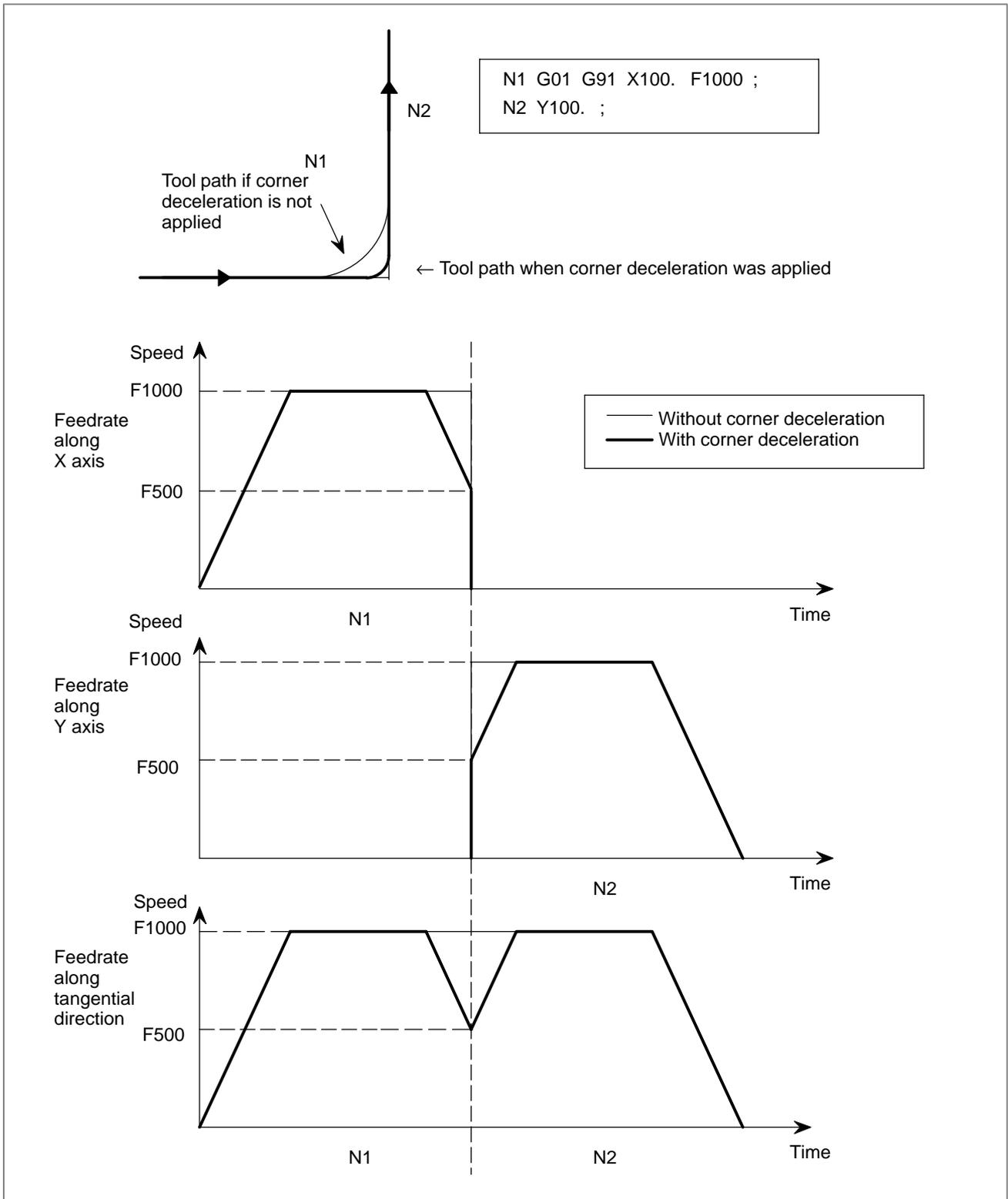
Different permissible feedrate differences can be specified for different axes. If a value is specified in parameter No. 1783, the permissible feedrate difference for each axis becomes valid. Deceleration at a corner is calculated for the axis for which the permissible feedrate difference is exceeded with the highest ratio of actual feedrate difference to permissible feedrate difference.
