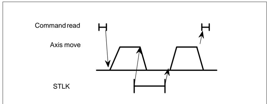
Fig. 2.5 (a) Block containing axis move commands only
