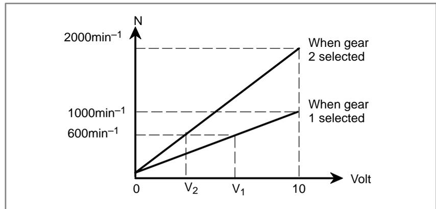
When spindle speed  $S=600$  is given,  $V_1$  (for G1) or  $V_2$  (for G2) is calculated inside the CNC and output to the machine side.
