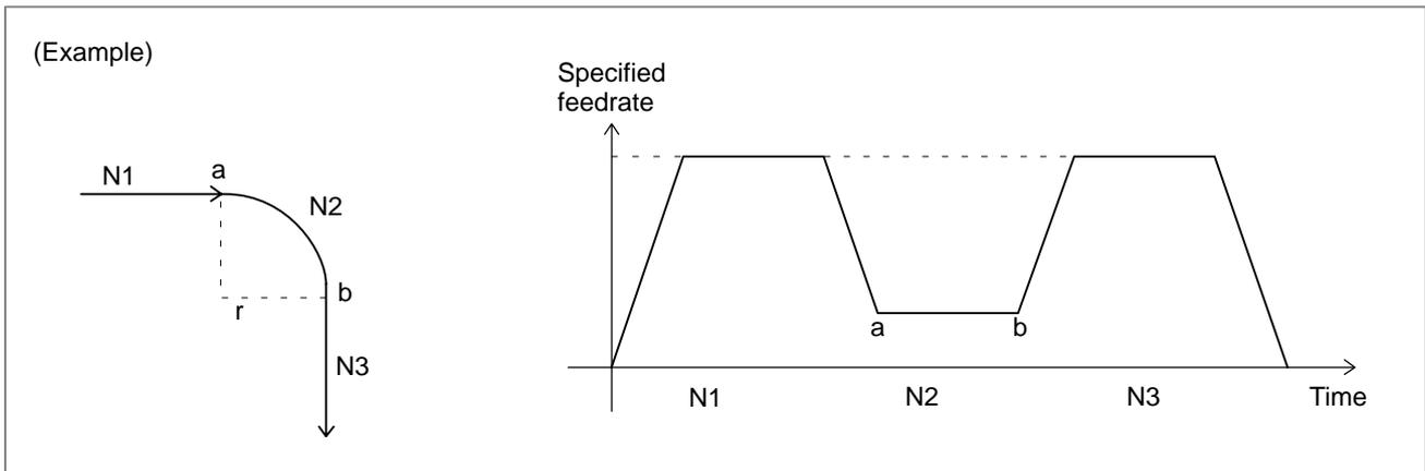
1732 Lower limit RVmin for feedrate clamping by arc radius
