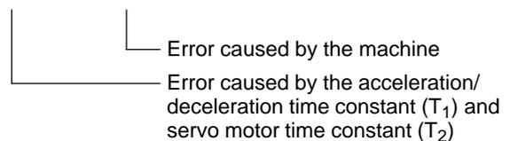
This function controls only the first term on the right side of expression 5. In other words, this function suppresses only the error caused by the acceleration/deceleration time constant ( $T_1$ ) and servo motor time constant ( $T_2$ ) to a certain level. This function does not control the error caused by the machine.
