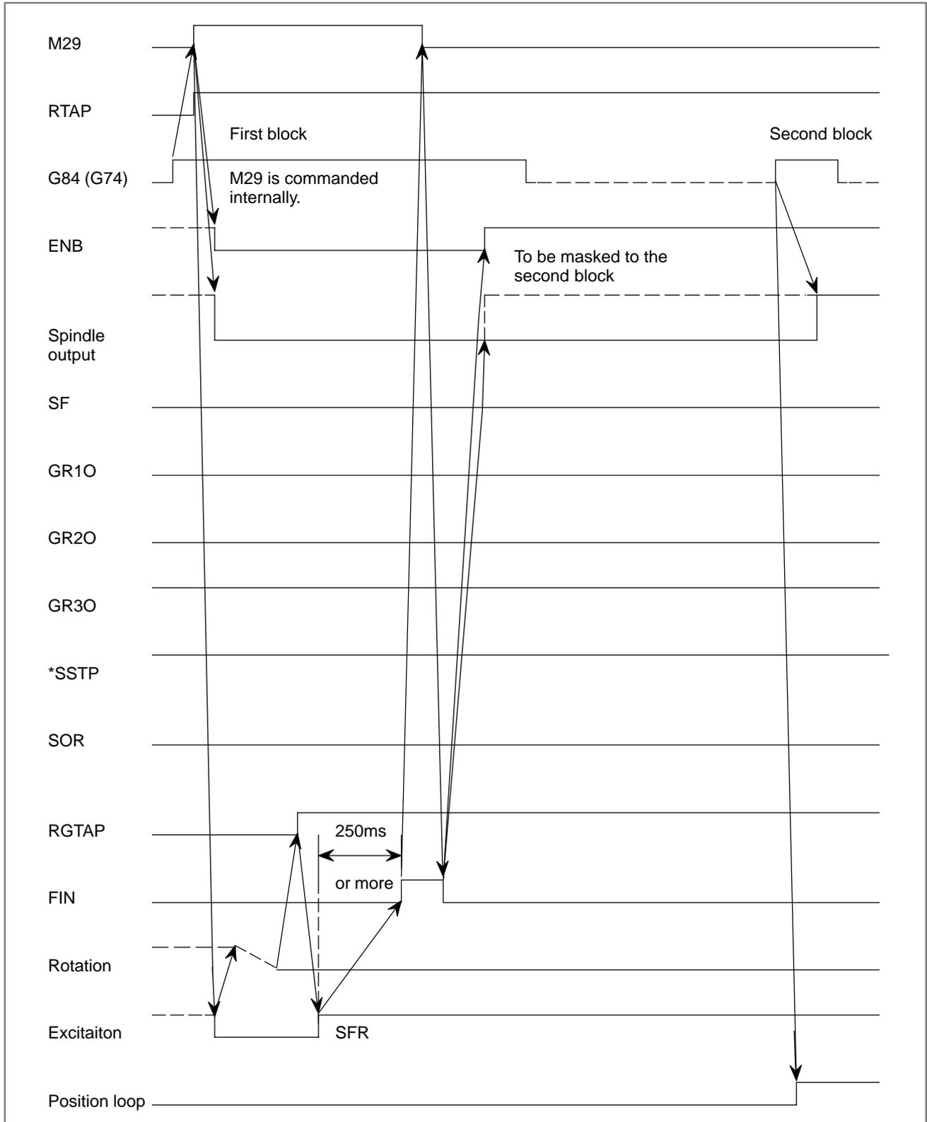
Fig. 9.10.7.3 (a) When gear-change is not performed
