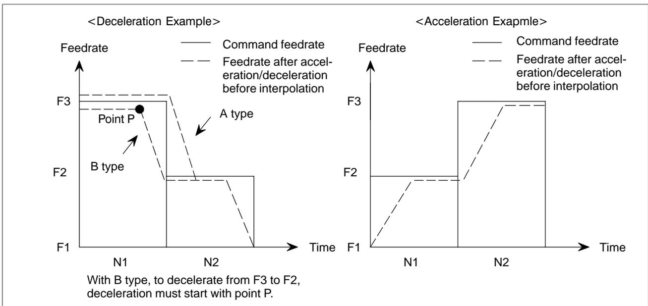
If an overtravel alarm occurs during linear acceleration/deceleration before interpolation, the movement is decelerated and stopped. As deceleration and stop are performed after the alarm occurs, the tool will overrun by an amount equal to the distance required for the deceleration. The actual overrun depends on the feedrate when the overtravel alarm occurs.
