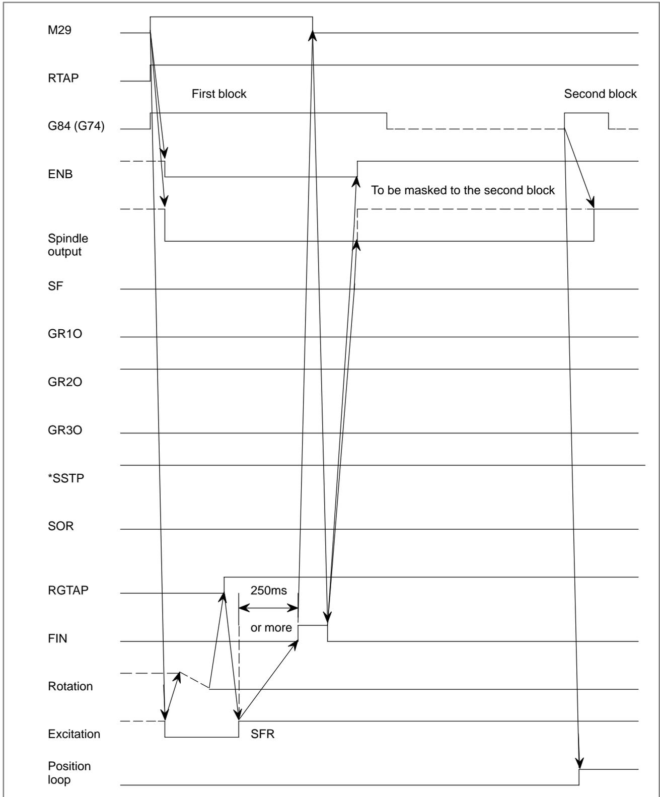
**Fig. 9.10.7.2 (a) When gear-change is not performed**
