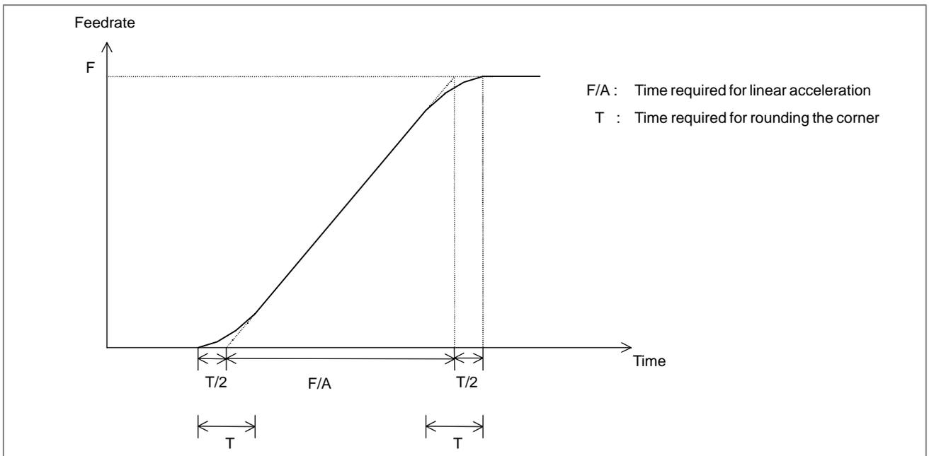
When the non-linear interpolation type is selected, movement is performed at the feedrate set in parameter No. 1420 with acceleration/deceleration set in parameter No. 1620. The corresponding value can be set in parameter No. 1621 to select bell-shaped acceleration/deceleration.
