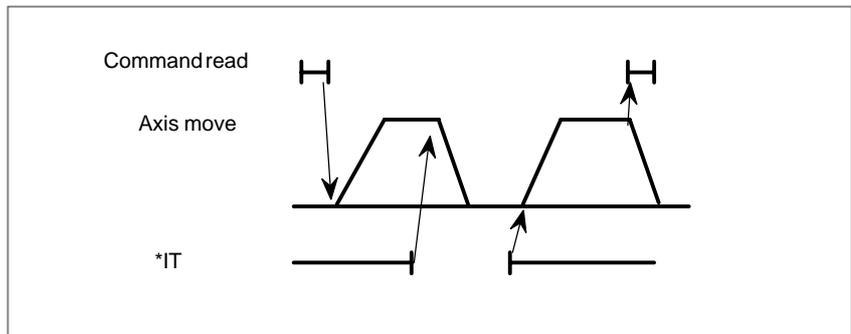
**Fig. 2.5 (c) Block containing axis move commands only (manual and automatic operation)**
