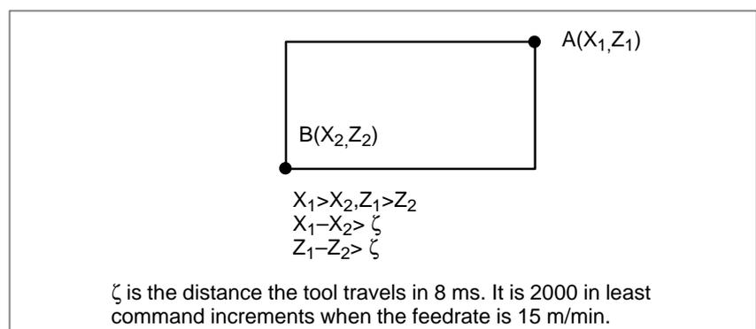
**Fig. 2.3.3 (e) Creating or changing the forbidden area using parameters (T series)**
