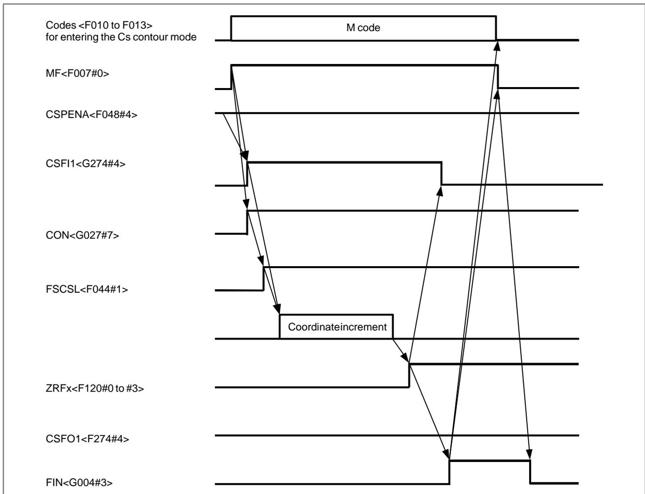
The Cs axis coordinate setup function is valid only during Cs contour mode. If the Cs axis coordinate setup request signal CSFI1 <G274#4> is set to '1' during any other mode, it is ignored.
