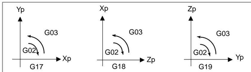
The end point of an arc is specified by address  $X_p$ ,  $Y_p$  or  $Z_p$ , and is expressed as an absolute or incremental value according to G90 or G91. For the incremental value, the distance of the end point which is viewed from the start point of the arc is specified with a sign.
