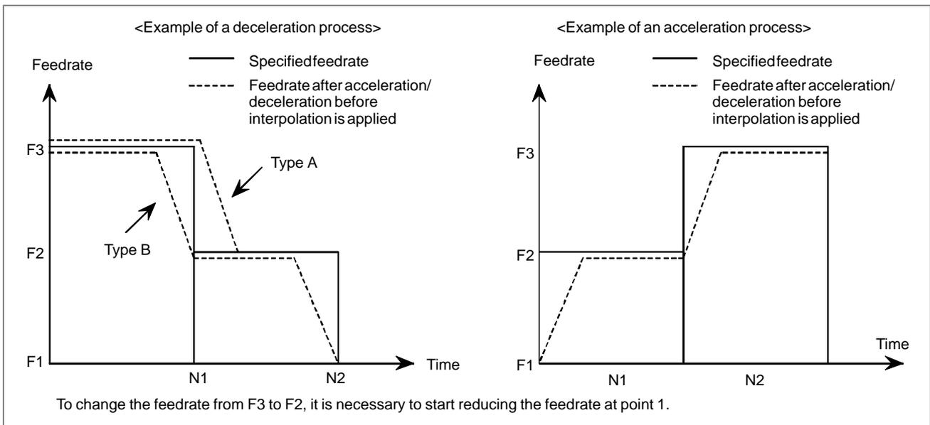
**BS2** The type of acceleration/deceleration after interpolation in cutting feed in advanced preview control mode is:
