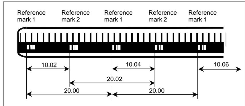
Fig. 4.8 (a) Sample linear scale with absolute addressing reference marks
