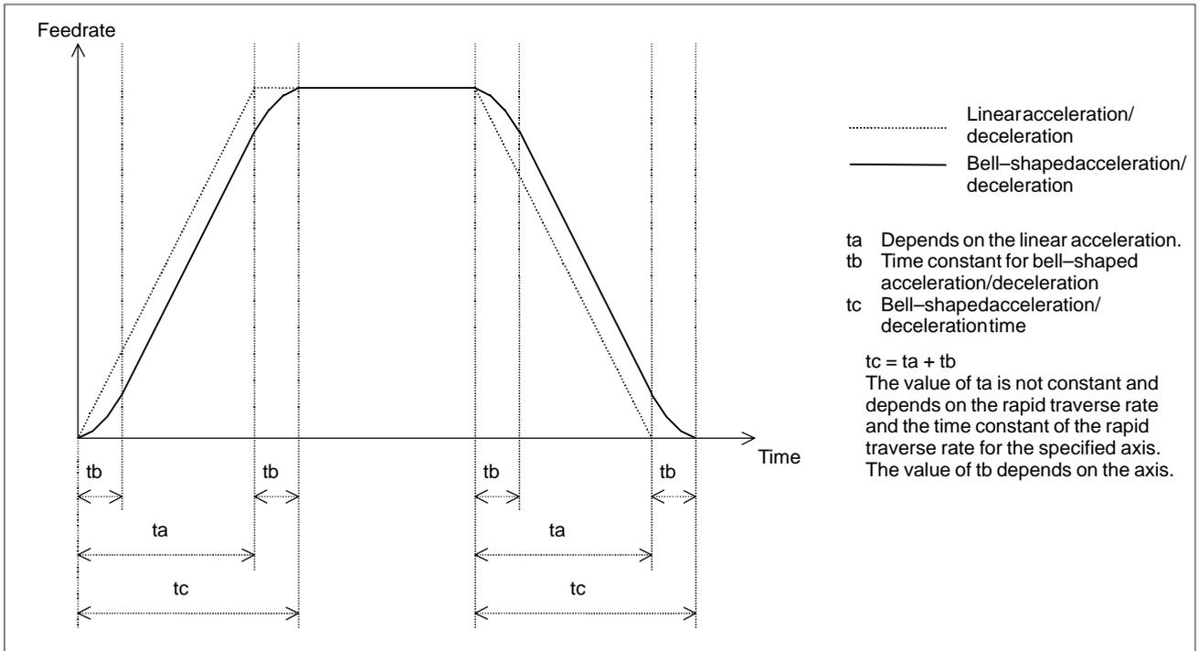
If the feedrate during movement is  $F$ , the acceleration for linear acceleration/deceleration is  $A$ , the time constant for bell-shaped acceleration/deceleration is  $T$ , the time required for acceleration/deceleration can be obtained as follows:
