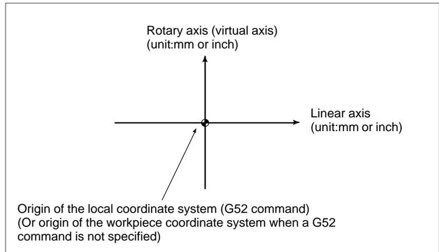
**Fig. 6.7 Polar coordinate interpolation plane**
