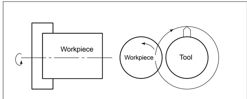
**Fig. 6.9 (a) Polygonal turning**
