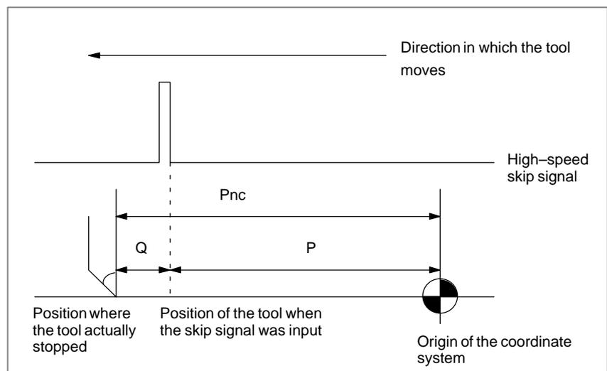
Pnc : Position where the tool actually stopped after the skip signal was input [mm/inch]
