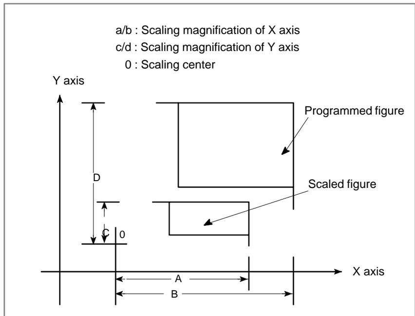
Fig. 11.11 (b) Scaling of each axis
