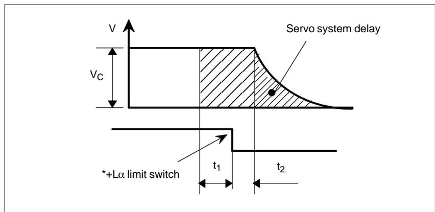
$$L_2 = V_C \left( t_1 + t_2 + \frac{T_S}{2} + T_S \right) \cdot \frac{1}{60000} \text{ [mm or inch]}$$
