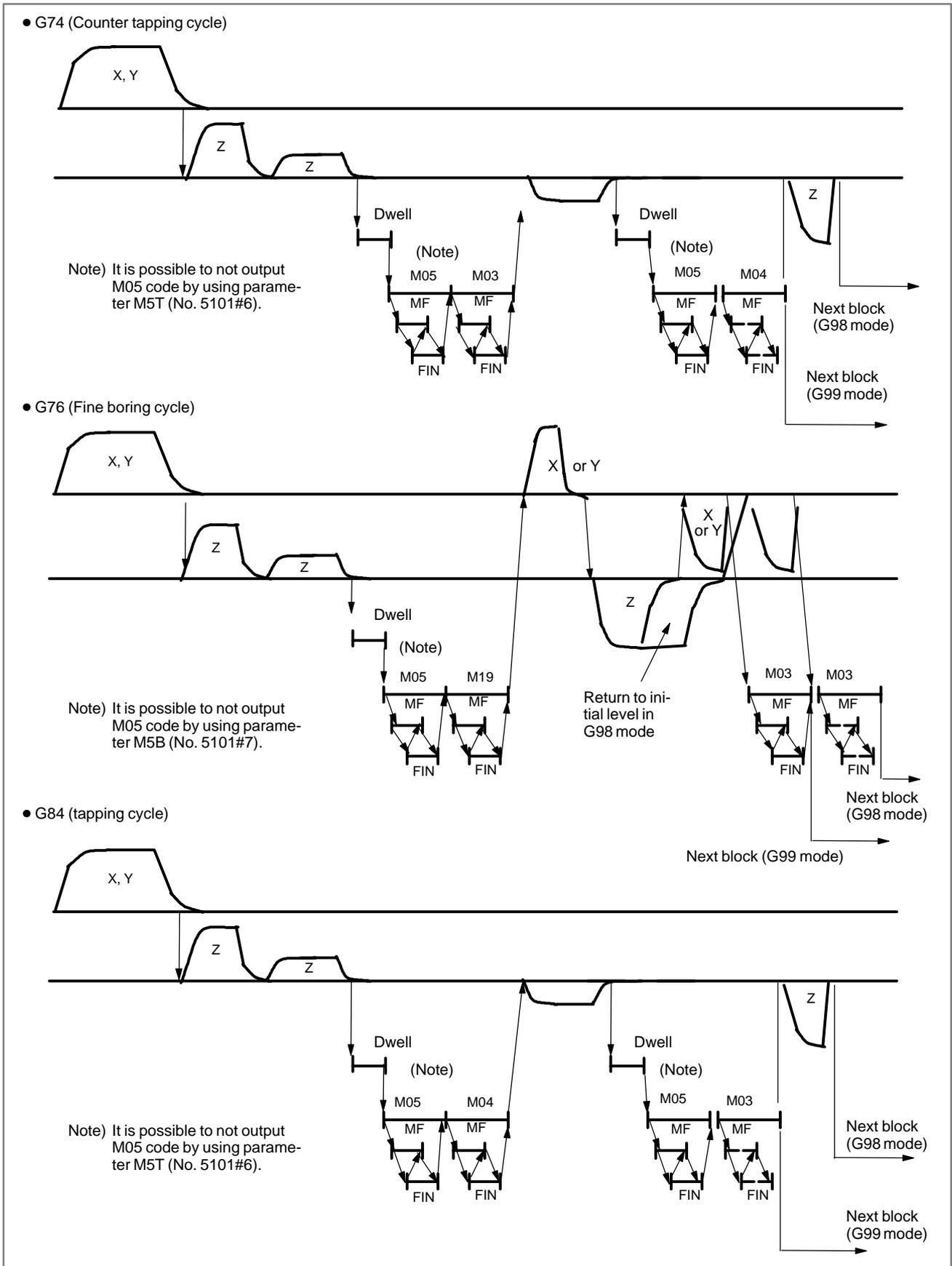
Fig. 11.6 (b) Canned cycle for M series (1/2)
