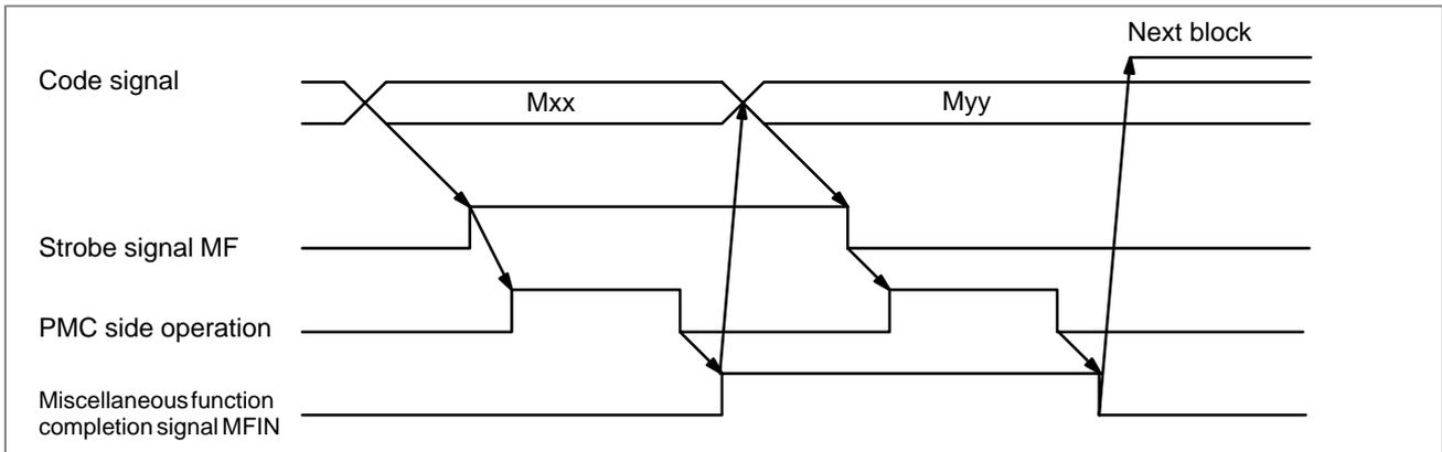
Fig. 8.4 (a) Timing chart of the high-speed system
