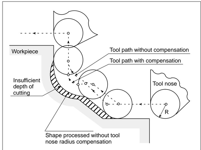
**Fig. 10.4.2 Tool path of tool nose radius compensation**
