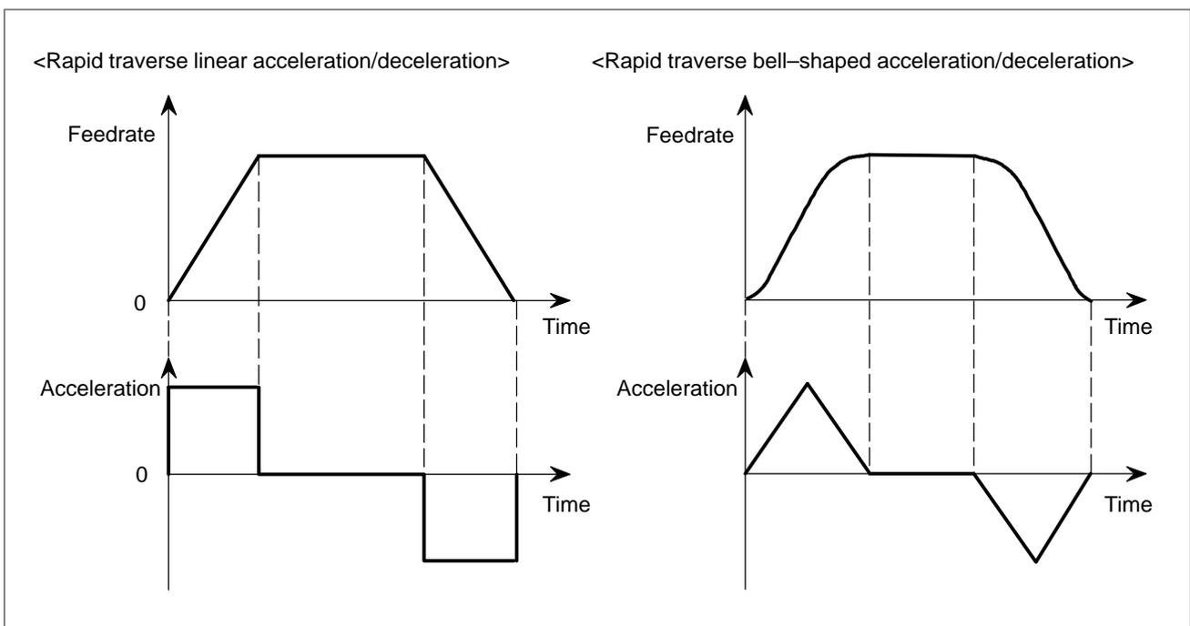
This function is enabled when the time constants for rapid traverse bell-shaped acceleration/deceleration  $T_1$  and  $T_2$  are specified in parameter Nos. 1620 and 1621, respectively.
