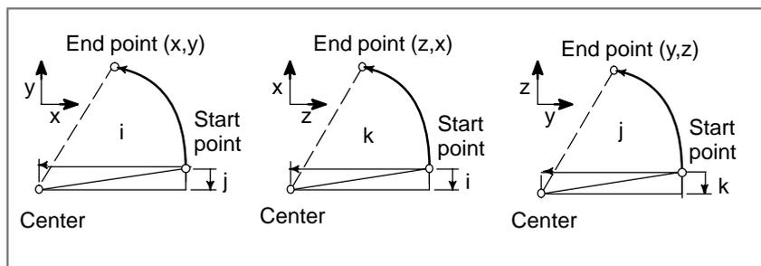
I0, J0, and K0 can be omitted. When  $X_p$ ,  $Y_p$ , and  $Z_p$  are omitted (the end point is the same as the start point) and the center is specified with I, J, and K, a 360° arc (circle) is specified.
