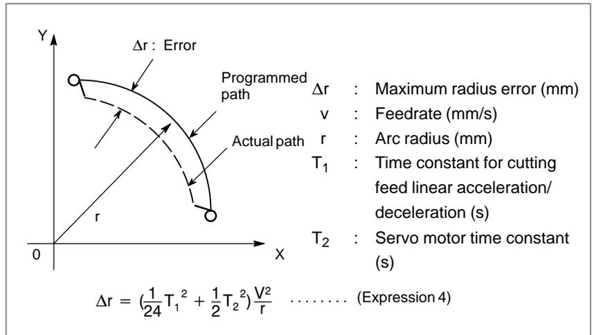
As can be seen from expression 4, expression 3 also holds for linear acceleration/deceleration after interpolation. Therefore, feedrate clamping by the arc radius is enabled.
