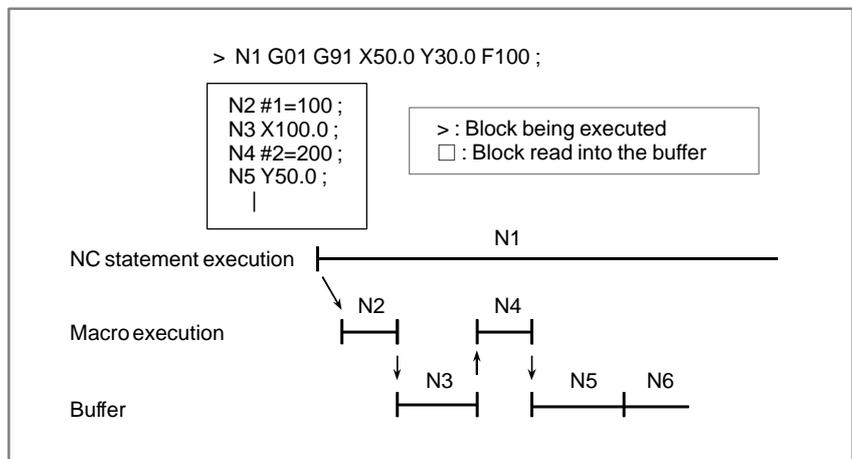
In the AI advanced preview control or AI contour control mode, multiple blocks are read in advance. So, during execution of N1, up to 40 blocks/20 blocks (0i) or 12 blocks (0i Mate) of NC statements are read into the buffer. The macro statements (N2, N4) are processed while N1 is being executed.
