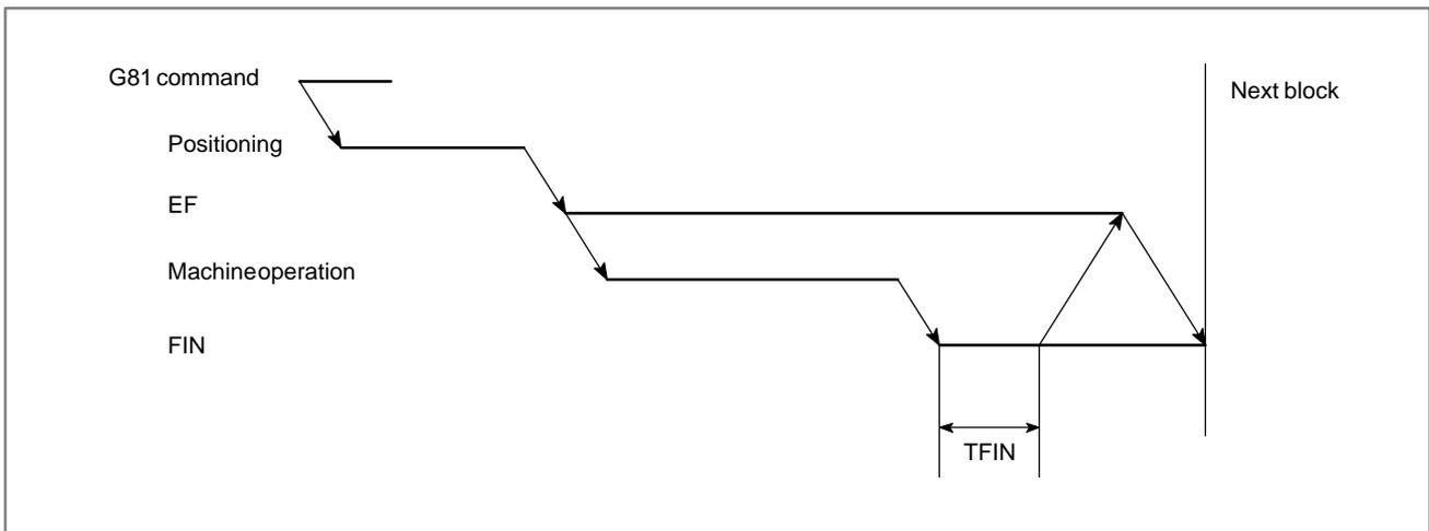
Fig. 11.7 Timing diagram of basic procedure
