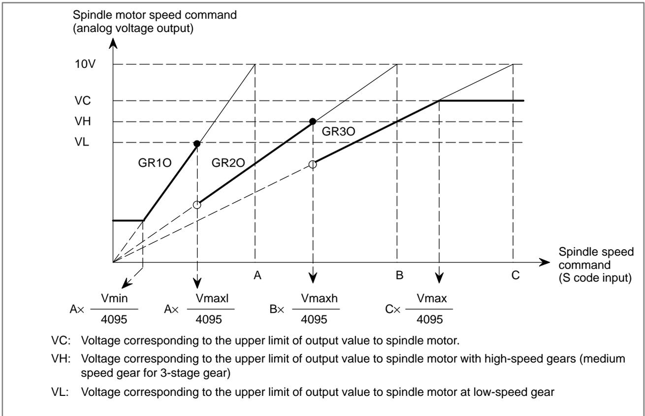
**Fig. 9.3 (c) M type gear change B**
