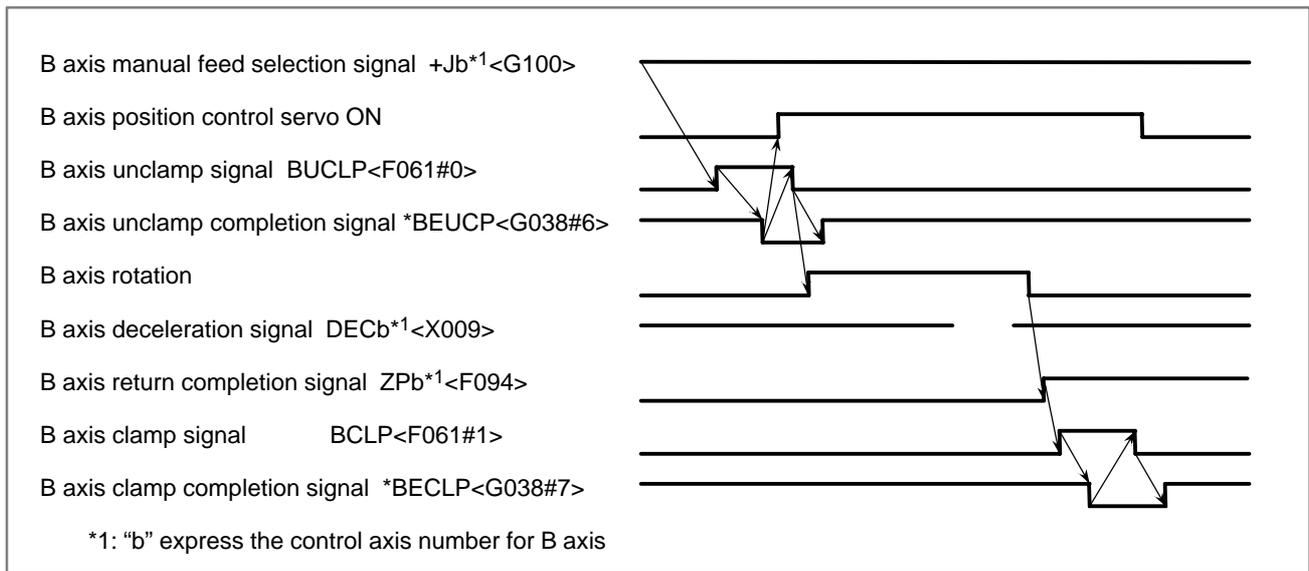
Fig. 11.10 (c) Manual reference position return of B axis (type A)
