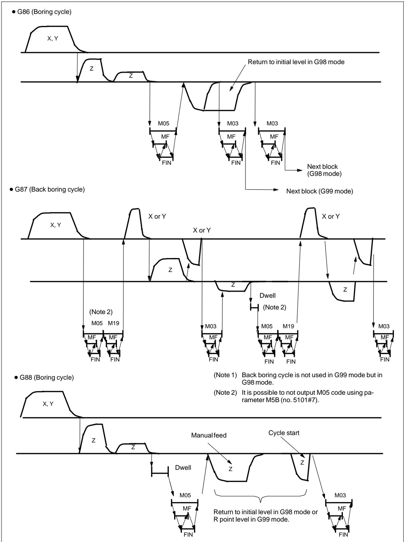
Fig. 11.6 (c) Canned cycle for M series (2/2)
