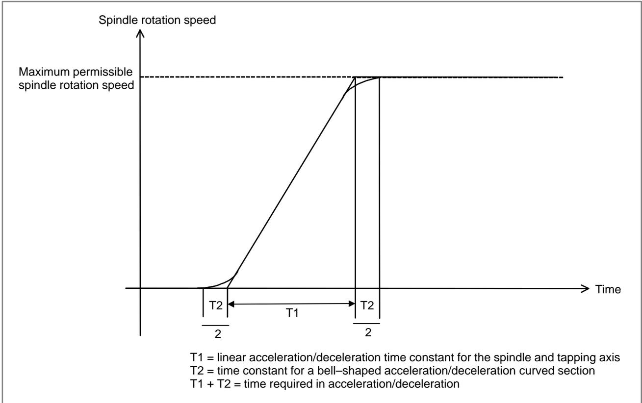
The actual linear acceleration/deceleration time constant, T1, for the spindle and tapping axis is determined according to the ratio of the maximum permissible spindle rotation speed to the actually specified value S. The bell-shaped acceleration/deceleration time constant for the curved section is not proportional to the actual S command. Instead, the bell-shaped acceleration/deceleration is kept constant (value specified in the parameter).
