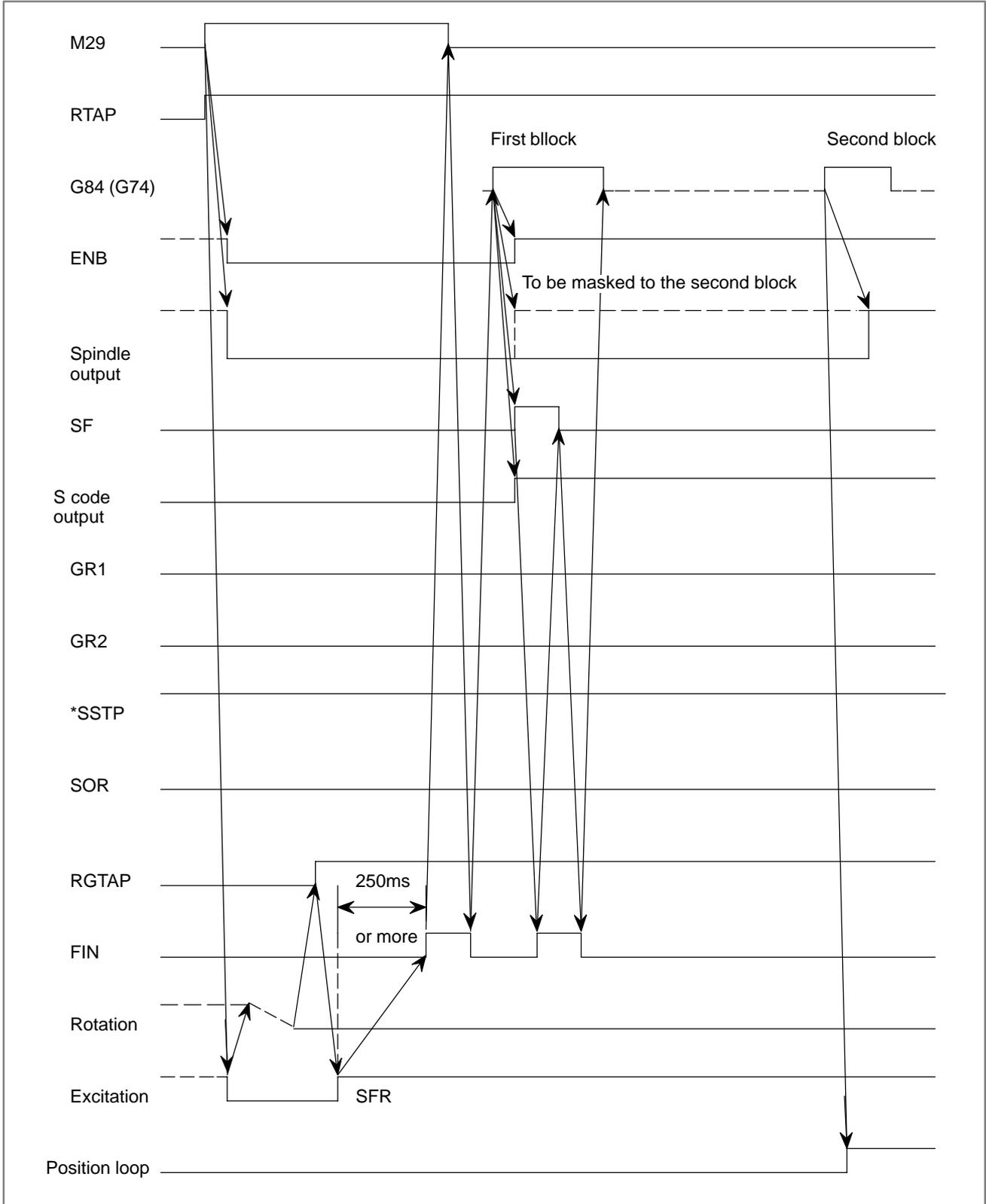
**Fig. 9.10.7.1 (c) Gear change is not performed**
