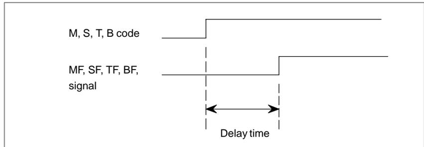
**Fig. 8.1 (a) Delay time of the strobe signal**
