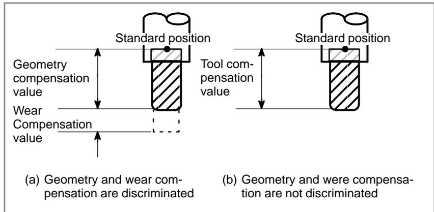
**Fig. 10.2 (a) Geometric compensation and wear compensation**
