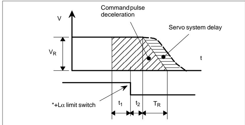
$$L_1 = V_R \left( t_1 + t_2 + \frac{T_R}{2} + T_S \right) \cdot \frac{1}{60000} \text{ [mm or inch]}$$
