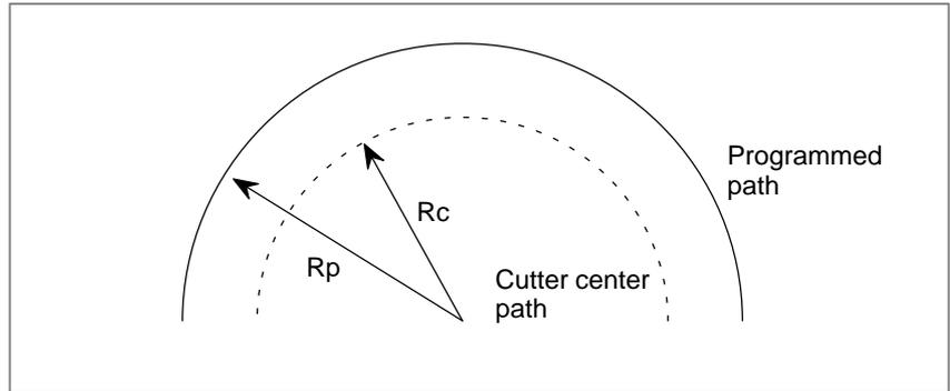
If  $R_c$  is too small in comparison with  $R_p$  so that  $\frac{R_c}{R_p} \approx 0$ , the cutter will stop. To prevent this, the minimum deceleration ratio (MDR) is set.
