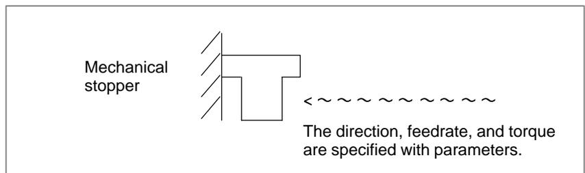
(B) After the tool strikes the mechanical stopper, the tool is withdrawn in the direction opposite to the butting direction, along the axis for a parameter-set distance.
