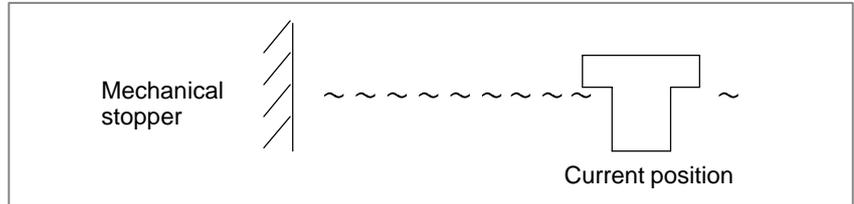
(A) The tool is moved along a specified axis with a limited torque until it butts against the mechanical stopper.
