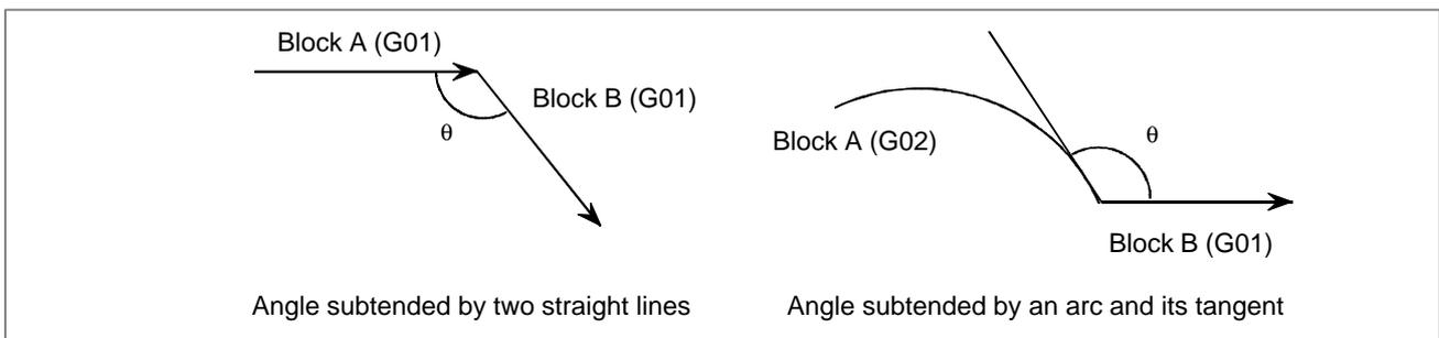
1780 Allowable speed difference for the speed difference-based corner deceleration function (for linear acceleration/deceleration before interpolation)
