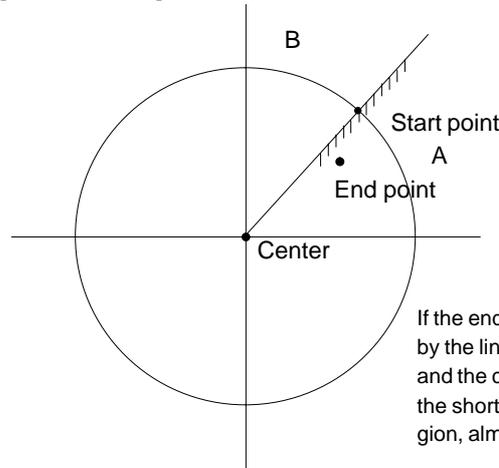
If the end point is in the A region separated by the line L drawn between the start point and the center, the movement is made along the shortcut. If the end point is in the B region, almost a single turn is made.
