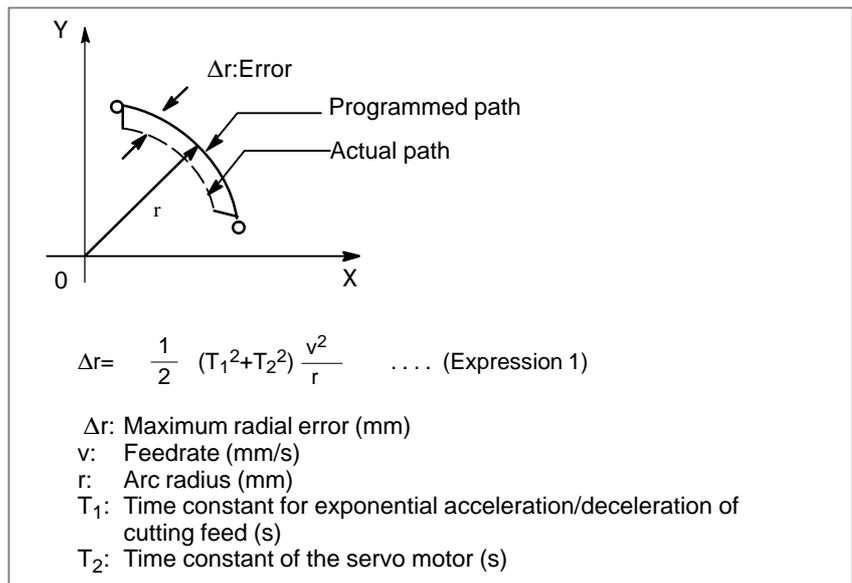
When actual machining is performed, radius  $r$  of the arc to be machined and permissible error  $\Delta r$  are given. Then, maximum allowable feedrate  $v$  (mm/min) is determined from the above expression.
