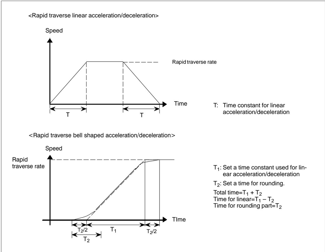
Set a time when rapid traverse override is 100% . When it is less than 100%, the total time is reduced (constant acceleration method).
