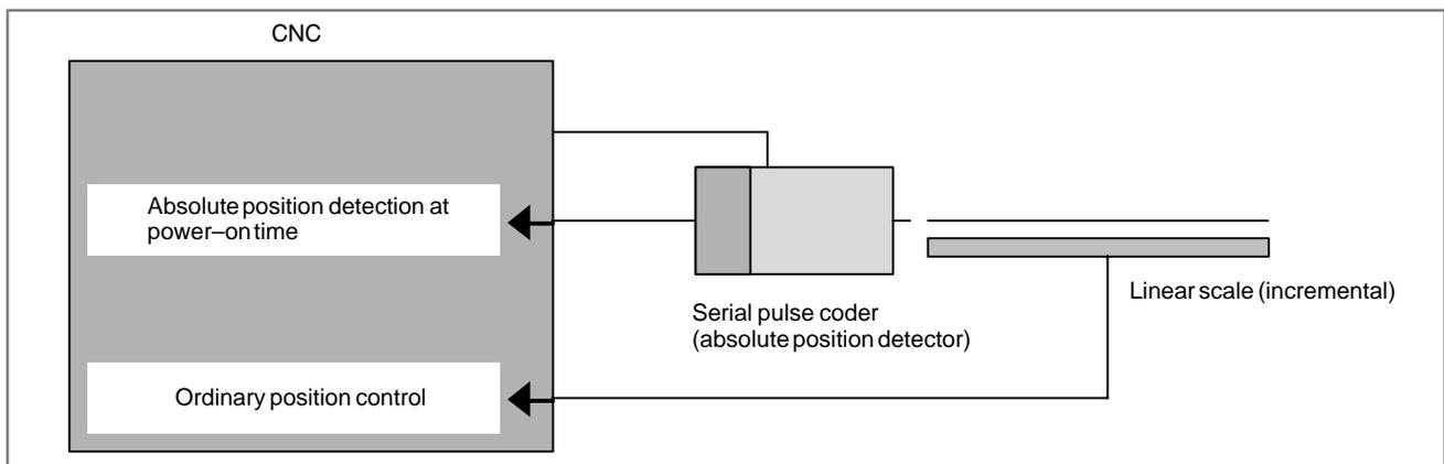
Fig. 1.4.4 System using tentative absolute coordinate system setting
