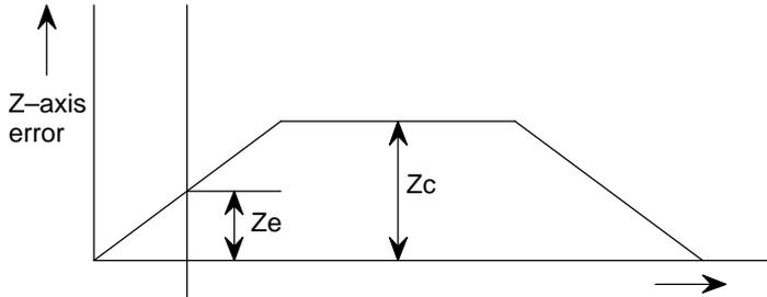
$$Z_c = \frac{\text{Speed}}{60} \times \frac{1}{\text{Gain}} \times \frac{1}{\text{Detection unit}} \times 10^2 \text{ (Theoretical value)}$$
