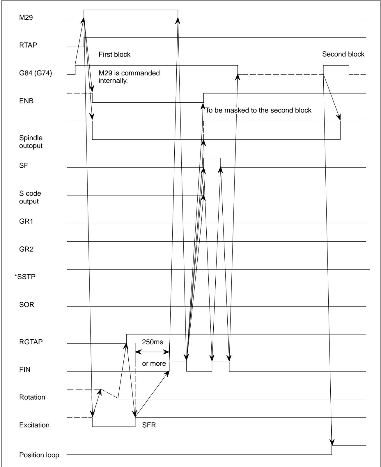
**Fig. 9.10.7.3 (c) When gear change is not performed**
