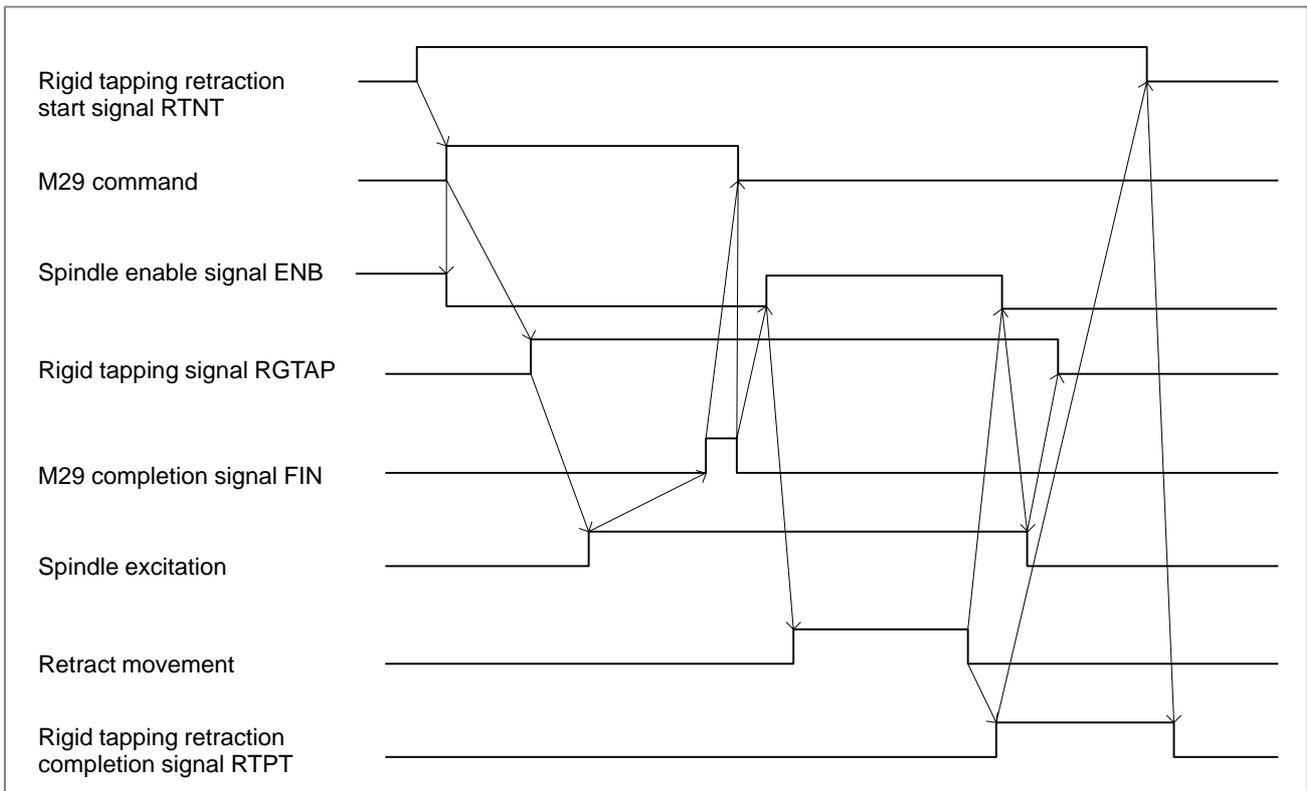
**Fig. 5.11 Start and completion time chart**
