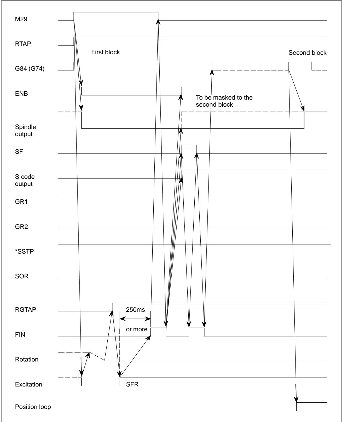
**Fig. 9.10.7.2 (c) When gear change is not performed**
