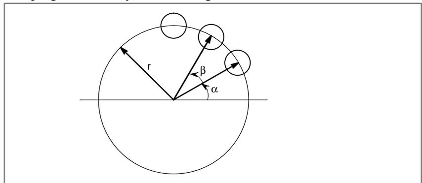
Bolt hole circles as shown in the above figure can be made easily.
