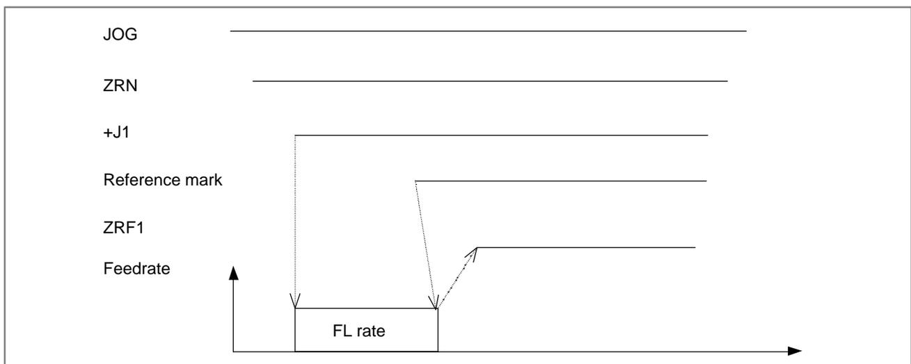
Fig. 4.7(c) Timing chart for reference position establishment
