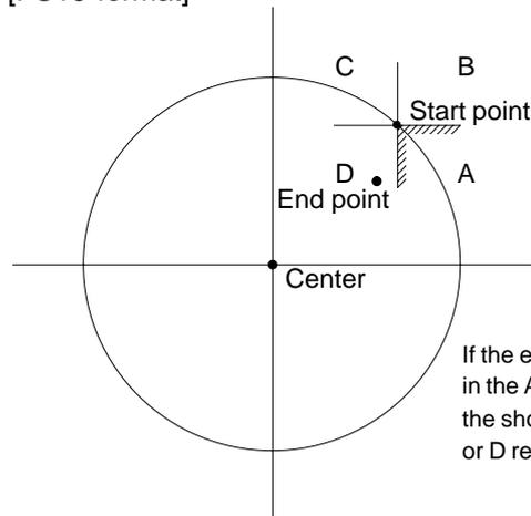
If the end point viewed from the start point is in the A region, the movement is made along the shortcut. If the end point is in the B, C, or D region, almost a single turn is made.
