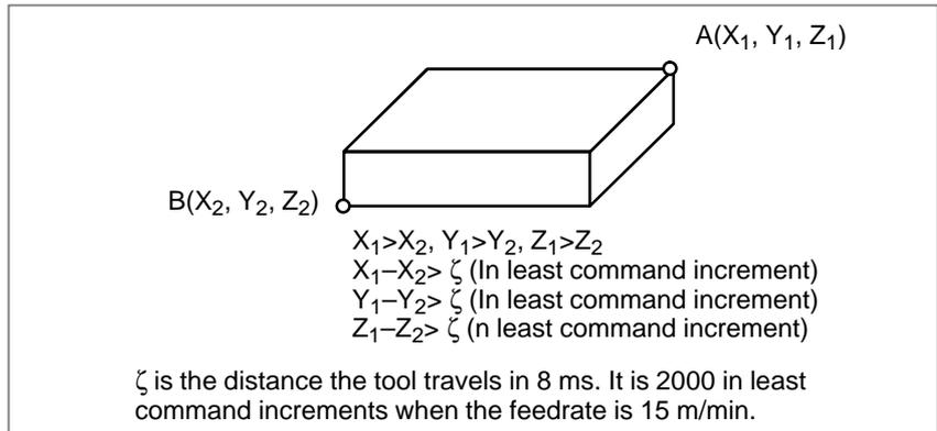
**Fig. 2.3.3 (f) Creating or changing the forbidden area using parameters (M series)**
