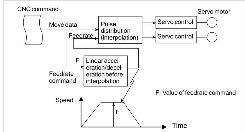
The function of linear acceleration/deceleration before interpolation increases or decreases the feedrate specified in the tangential direction.
